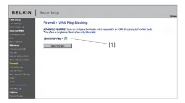
To turn off the ping response, select "Block ICMP Ping" [1] and click "Apply Changes". The Router will not respond to an ICMP ping.
